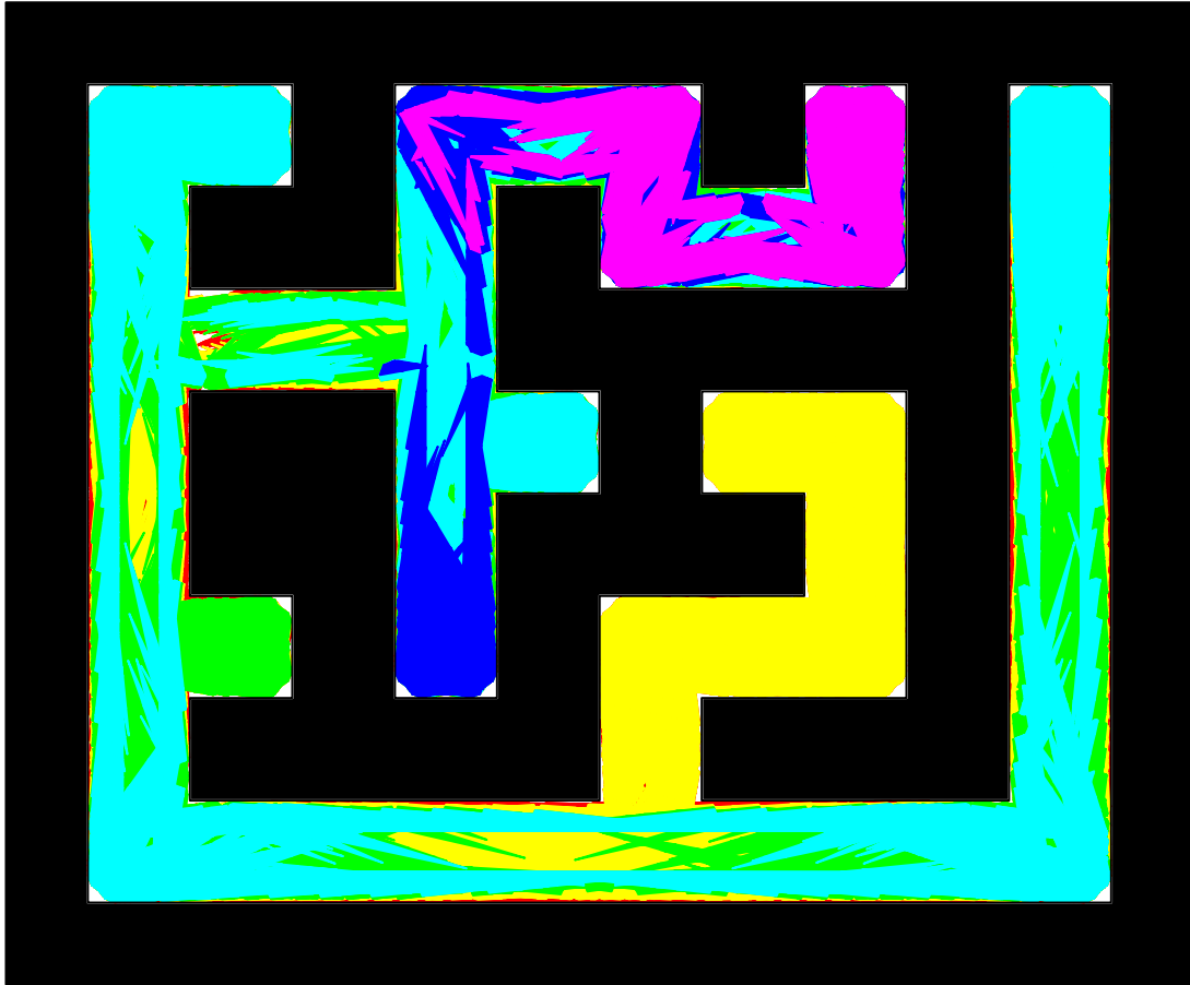
Figure 5.9 An office-like environment presenting both challenges in navigation and coverage. The robot begins in the third convex vertex from the right in the top-most section of the map and loses the ability to connect its starting nodes with the rest of the environment nodes when \theta_{\max} is \pm 3 .
