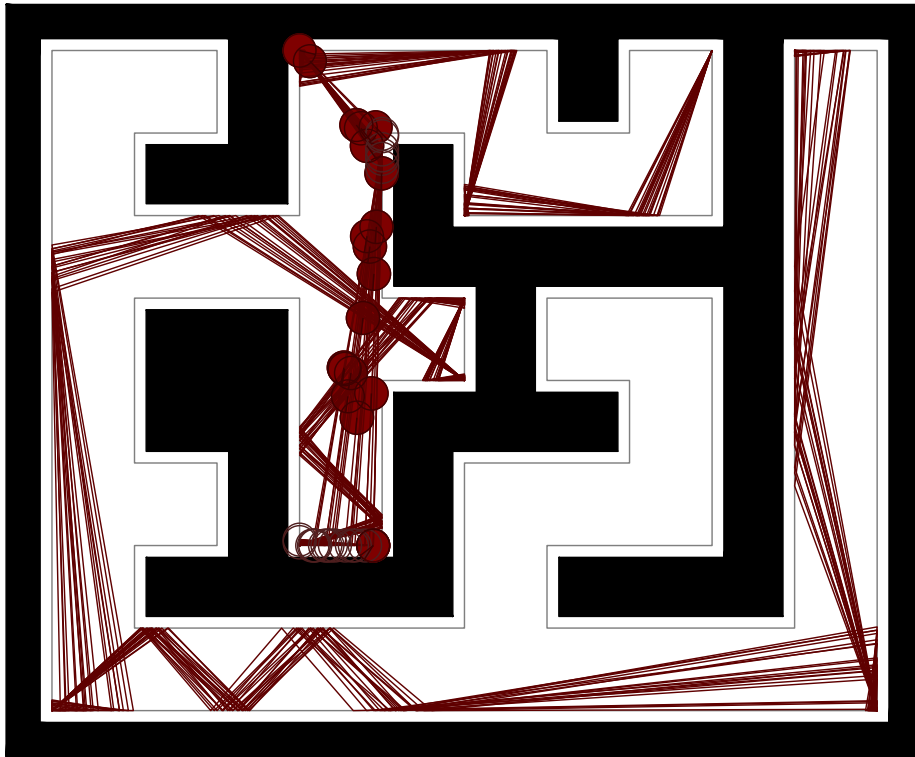
Figure 2.4 A plan generated using the discretized environment from Figure 2.3. The figure shows 20 simultaneous simulations of a robot executing that plan. [72]
