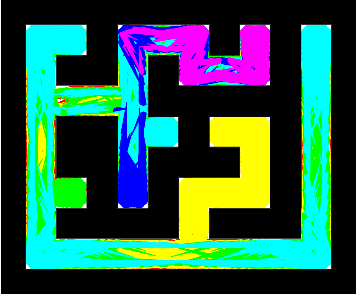
Figure 1.4 A maze-like environment. Our algorithm generates a plan that is guaranteed to cover the portions of this environment. Results from several runs of the algorithm, showing the region guaranteed to be covered by the approach for error bounds ranging from 0.5 degrees to 3 degrees of error on each motion, are shown. For example, the cyan shaded region is the portion of the environment covered by a plan generated by our algorithm for a robot that may experience up to 2 degree of error with each of its motions. The red region (largely occluded by other layers) is the result under a 0.5 degrees per motion error bound.
