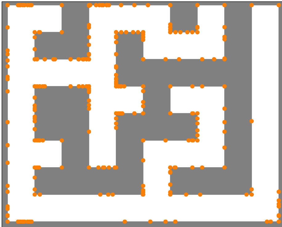
Figure 2.3 An environment environment discretized for blind navigation with corner-finding. [72]
